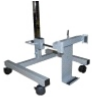
Detail of bilateral clamp and low reach of cassette holder.
