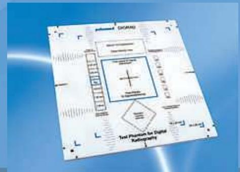
Test phantom per German standards (DIN 6868/58 and DIN 6868/13) for acceptance and constancy tests of digital radiography equipment (e.g. storage phosphor or full digital).
