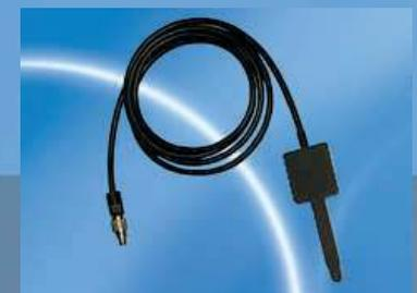
Fits the ALPHAplus Dosimeter for the constancy test of digital and analog X-ray-equipment (direct radiography and fluoroscopy; not for dental or mammography systems) Because of its shape the sensor is suitable for insertion into the patient-equivalent-filter for use with near-the-tube measurements as well as an external sensor. Energy range: 50kV - 155kV Effective dose range: 0,1mGy/s - 500mGy/s
